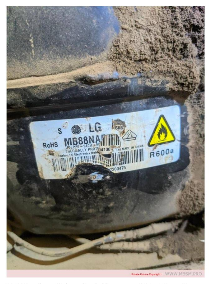
The **R600a refrigerant** further confirms that this compressor is intended for smaller, energy-efficient cooling systems.
