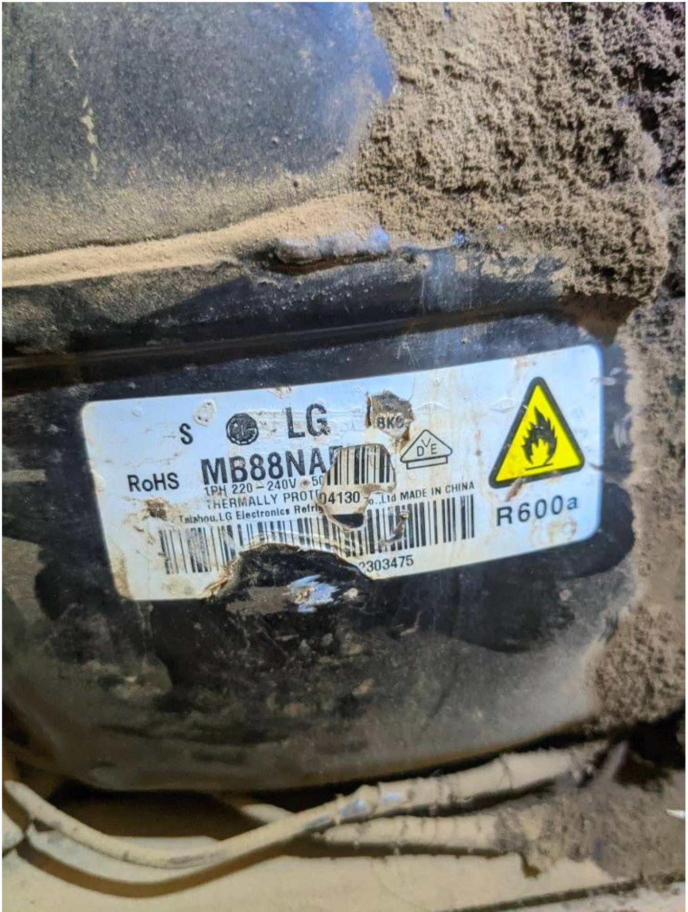
File Pdf, Mbsm.pro, Compressor, Lg, Lbp, MB88NA, 151 w, 1/5 hp, r600a, 1ph-220v-50hz
