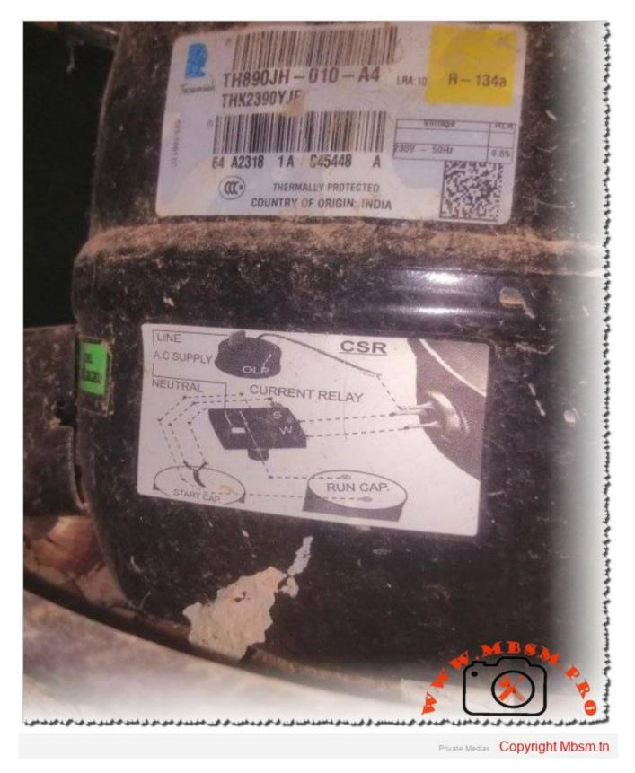
pdf, Mbsm.pro, Compressor, THK2390YJE, LBP, 1/3 hp, R134a, Freezing, Tecumseh Compressor
