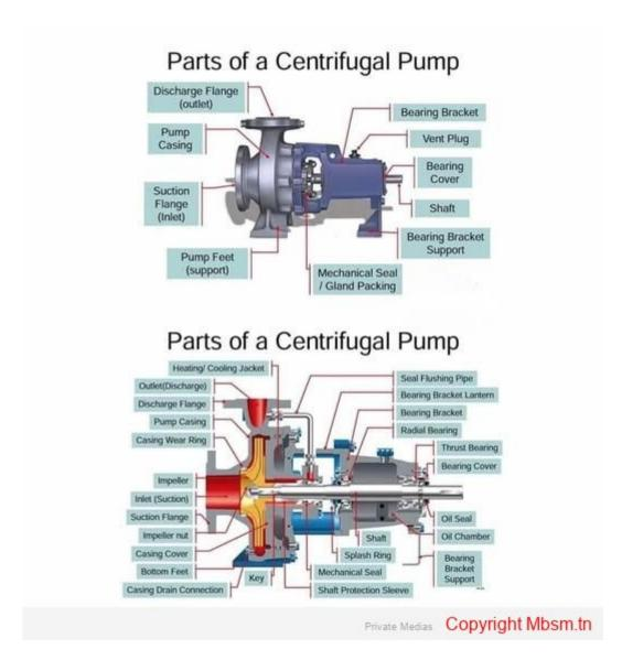
Centrifugal pumps are widely used devices for moving fluids, and they consist of several critical components that work together to perform this function. Here are the main parts of a centrifugal pump:
