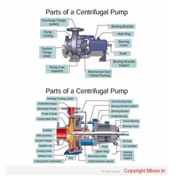
Centrifugal pumps are widely used devices for moving fluids, and they consist of several critical components that work together to perform this function. Here are the main parts of a centrifugal pump:
