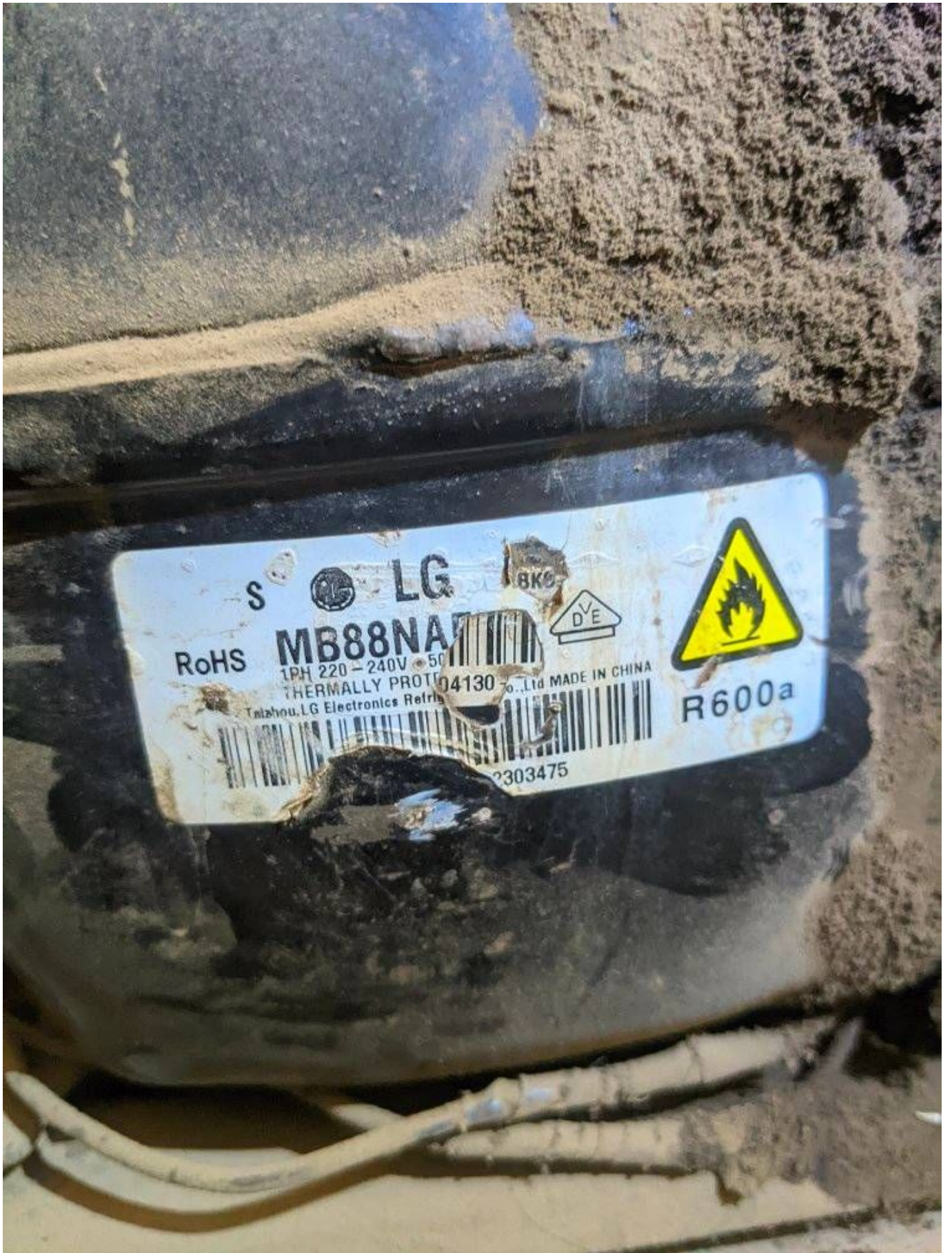
File Pdf, Mbsm.pro, Compressor, Lg, Lbp, MB88NA, 151 w, 1/5 hp, r600a, 1ph-220v-50hz
